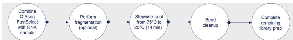
**Figure 1. QIAseq FastSelect –5S/16S/23S workflow.**
