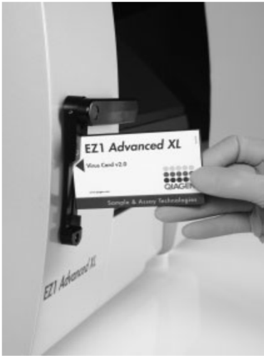
Figure 1. Ease of protocol setup using EZ1 Advanced XL Cards. Inserting an EZ1 Card, containing a protocol, into the EZ1 Advanced XL instrument.
