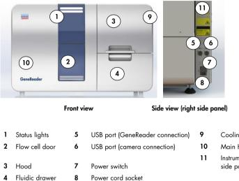
Cooling air outlet (back of instrument)
