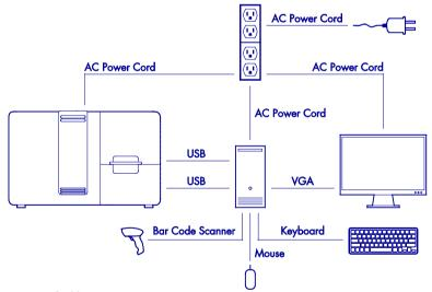
Diagram of cable connections
