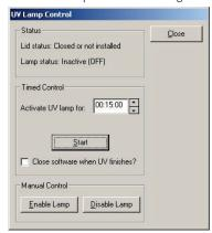
Lid status Indicates whether the instrument lid is **Closed or not installed** or **Open**.
