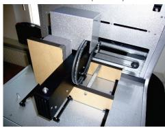
2. Move the pipetting head to the right and remove the transport lock from the worktable.
