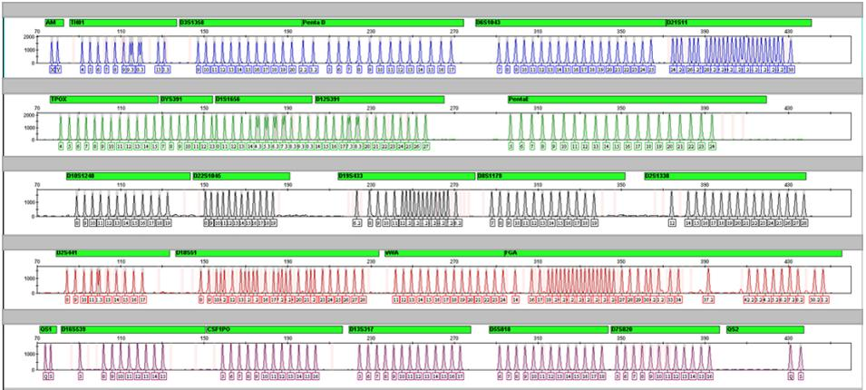
**Figure 6. Electropherogram of the allelic ladder 26plex analyzed on an Applied Biosystems 3500xL Genetic Analyzer.** The allelic ladder contains 2 alleles for each quality sensor (QS1 and QS2). This allows automated calling of the QS peaks for sample analysis.
