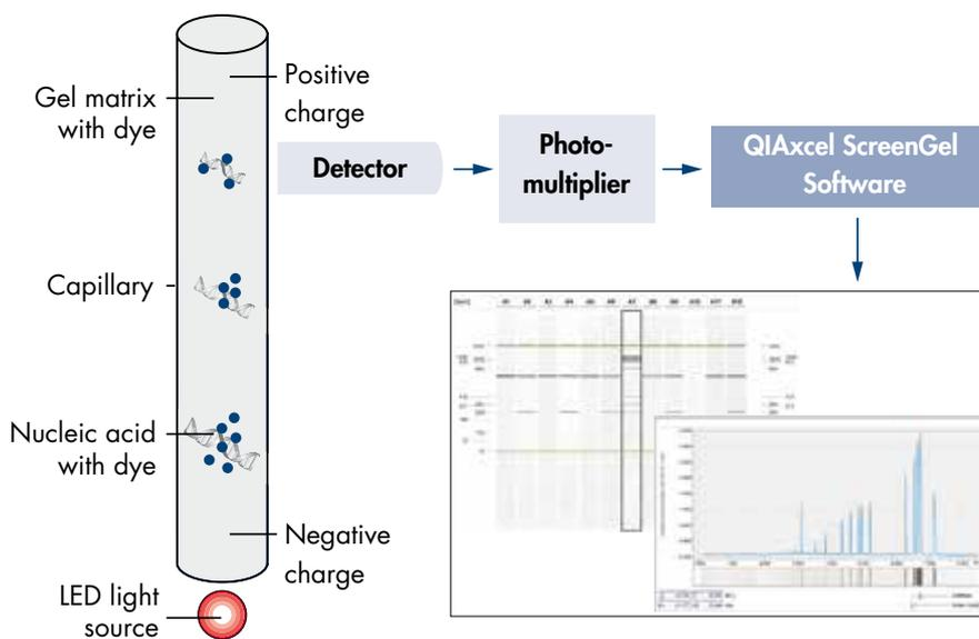
**Figure 11. QIAxcel Advanced process.** Nucleic acid molecules are size separated by applying a current to a gel-filled capillary, and detected as they migrate toward the positively charged terminus. The signal data pass through a photomultiplier and are converted to an electropherogram and gel image by the QIAxcel ScreenGel Software.
