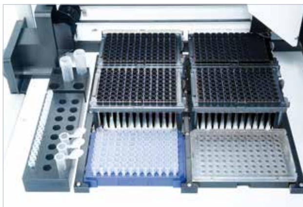
Figure 9. QIAgility instrument and deck layout.
