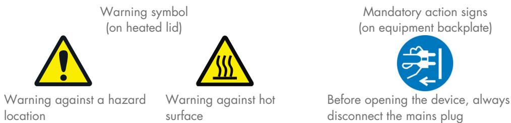
The following notice sign is attached to the rear of the QIAquant 384:
