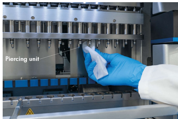
Figure 181. Cleaning the EZ2 Connect piercing unit.
