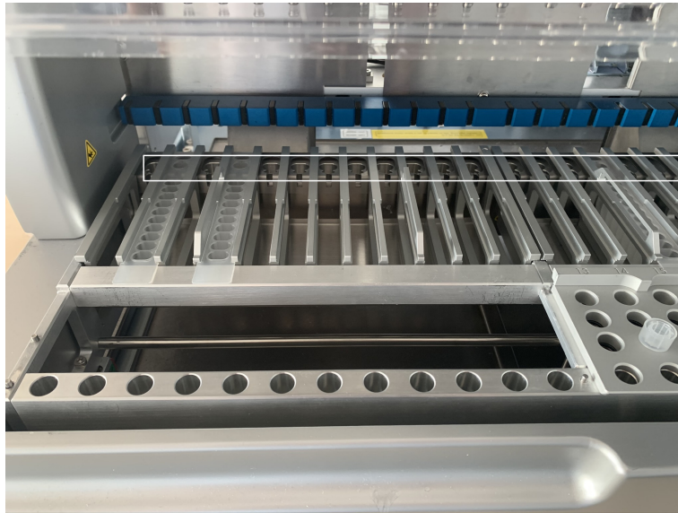
Figure 17. Heatable positions in the cartridge rack (highlighted by white frame).
