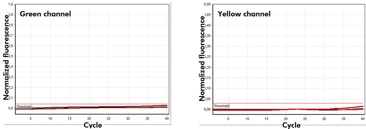
**Figure 3. The PCR is inhibited.** No amplification of the three samples in the green channel (left) or the internal control in the yellow channel (right). All curves lie along the baseline and do not exceed a preset threshold.
