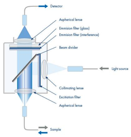
Figure 2. Schematic structure of the Epi Fluorescence Photometer.
