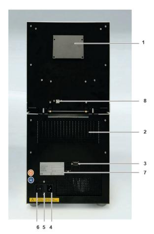
Figure 4. QIAquant 96 rear view. 1: Ventilation for fluorescence spectrometer, 2: ventilation grille at the thermal cycler, 3: service connection, 4: mains connection, 5: fuse holder for instrument fuses, 6: mains switch, 7: type plate, 8: USB port for PC connection.
