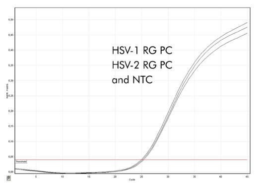
Figure 12. Detection of the internal control (IC) in fluorescence channel Cycling Yellow with simultaneous amplification of the positive controls (HSV-1 RG PC and HSV-2 RG PC). NTC: No template control (negative control).
