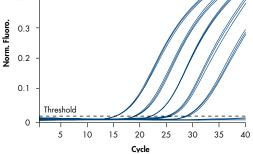
Figure 3. Highly reproducible assay setup. A series dilution of leukocyte cDNA (100 ng to 0.01 ng) was performed A manually and S using the <u>QIAsymphony AS</u>. GAPDH was amplified from these dilutions, using the <u>Rotor-Gene Q</u> and the <u>QuantiFast® Probe PCR Kit</u>. Reactions were set up in replicates of 4 in Strip Tubes.
