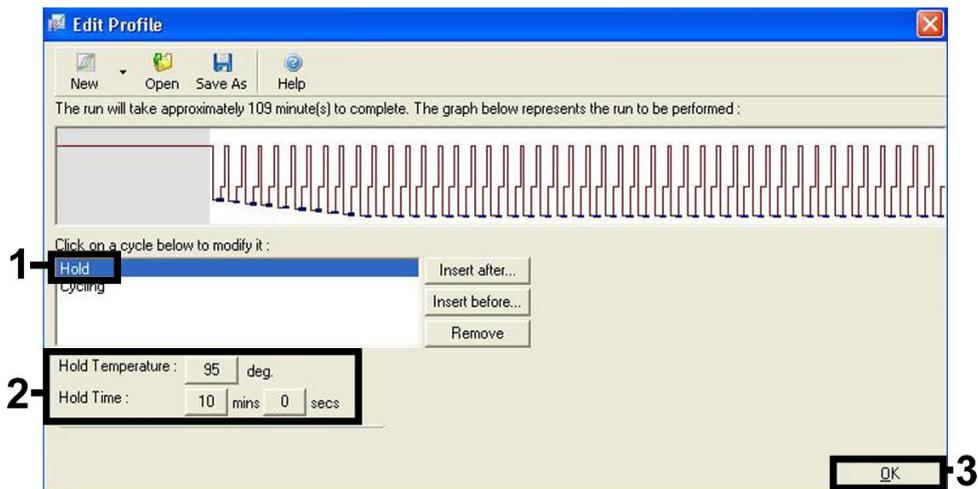
Figure 4. Initial activation of the hot-start enzyme.
