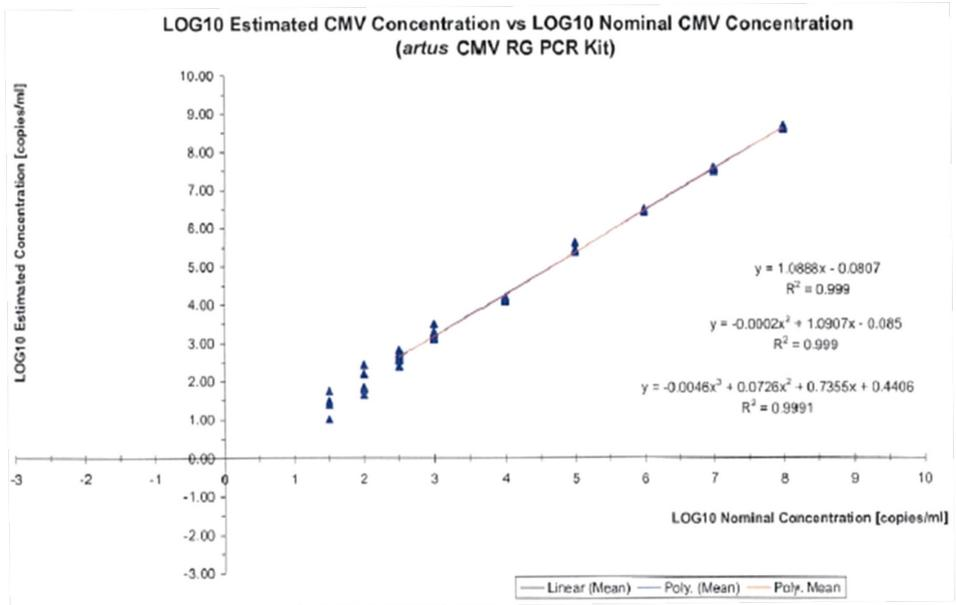
**Figure 12. Polynomial regression of dataset of *artus* CMV RG PCR Kit in consideration of the purification (EZ1 DSP Virus Kit) on the EZ1 Advanced XL instrument. Linear, quadratic, and cubic regression models are included.**
