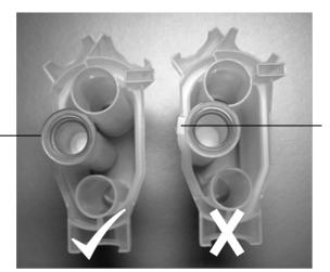
Column lid removed incorrectly. Part of lid still attached to PSC.
