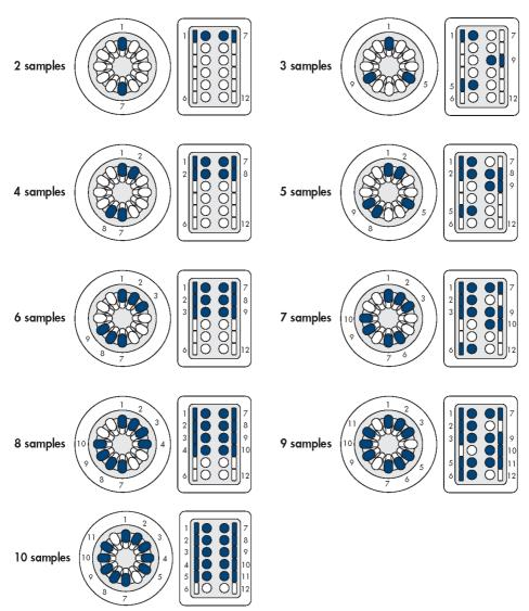
**Figure 22: Loading the centrifuge and shaker.** Centrifuge and shaker positions are shown for processing from two (2) to ten (10) samples. One (1) or 11 samples cannot be processed. For processing 12 samples, all centrifuge and shaker positions are loaded (image not shown).
