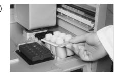
Figure 17: Loading the reagent bottle rack. [A] Schematic of positions and contents of bottles in the reagent bottle rack. [B] Loading the rack onto the QIAcube Connect MDx.
