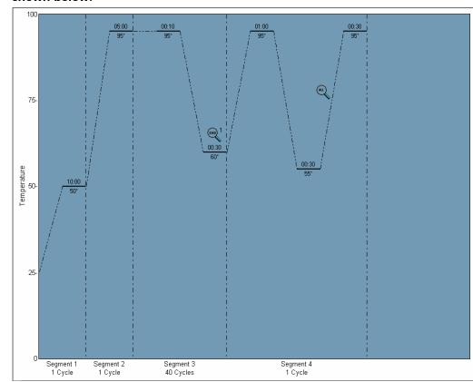
1. Launch the software and set up the parameters for RT-PCR and melting curve analysis as shown below.
