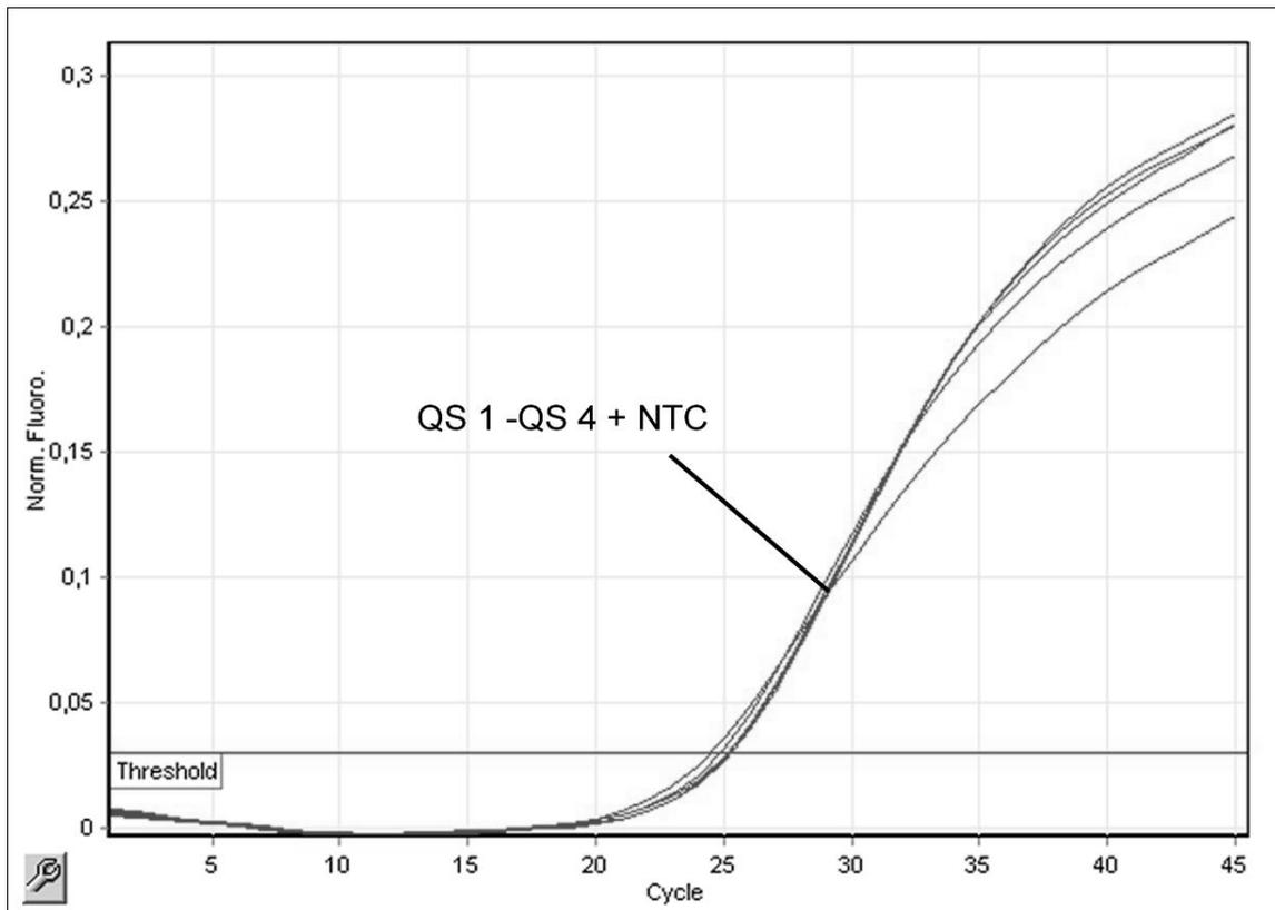
**Figure 19. Detection of the internal control (IC) in fluorescence channel Cycling Yellow with simultaneous amplification of the quantitation standards (CMV QS 1–4). NTC: No template control (negative control).**
