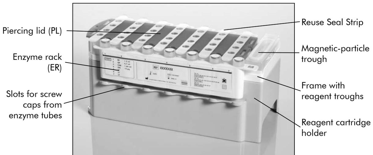
**Figure 3. QIAasymphony reagent cartridge (RC).** The reagent cartridge (RC) contains all reagents required for the purification procedure.
