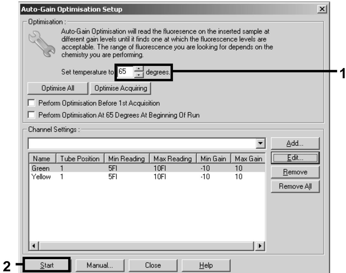
Figure 10. Adjusting the fluorescence channel sensitivity.
