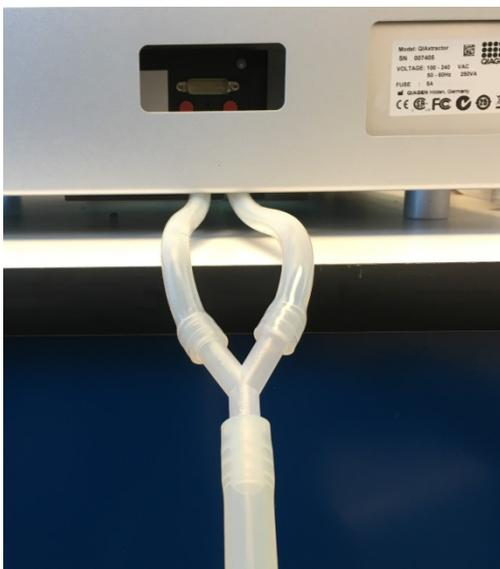
6. Plug the Polycap filter into the correct opening on the vacuum station.
