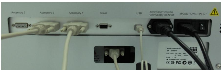
12. Connect one end of the AC power cord (standard 3-wire IEC mains cable) to the power connector of the vacuum control station. Connect the other end to the AC power outlet.
