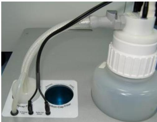
9. Screw the Carbon-Cap filter into place in the correct opening on the vacuum station. Be sure to position the filter with the labeling upside down
