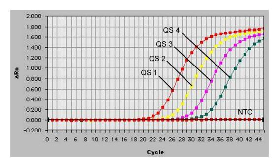
Fig. 25: Detection of the *Quantitation Standards* (*EBV LC/RG/TM QS 1 - 4*) by measurement of the FAM fluorescence signal (*ABI PRISM® 7700 SDS*). NTC: non-template control (negative control).
