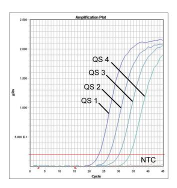
Fig. 27: Detection of the *Quantitation Standards* (*EBV LC/RG/TM QS 1 - 4*) by measurement of the FAM fluorescence signal (*ABI PRISM® 7900HT SDS*). NTC: non-template control (negative control).
