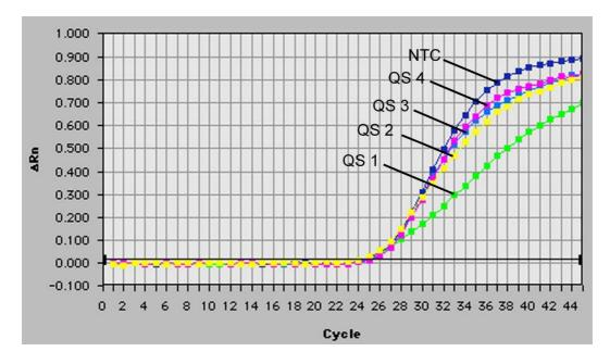
Fig. 26: Detection of the *Internal Control* (*IC*) by measurement of the VIC fluorescence signal (*ABI PRISM®* 7700 SDS) with simultaneous amplification of the *Quantitation Standards* (*EBV LC/RG/TM QS 1 - 4*). NTC: non-template control (negative control).
