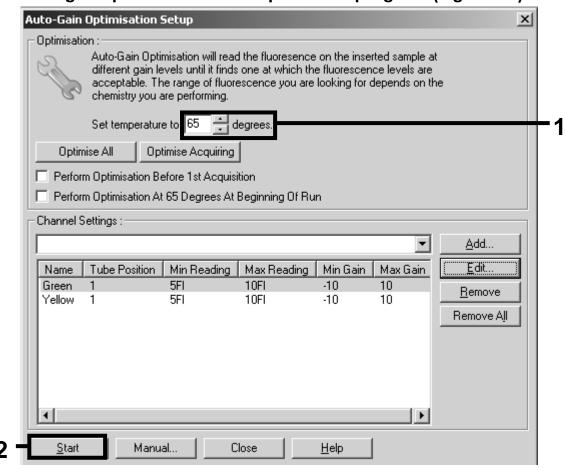
Figure 10. Adjusting the fluorescence channel sensitivity.
