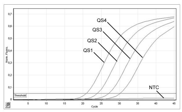
Figure 18. Detection of the quantitation standards (CMV QS 1–4) in fluorescence channel Cycling Green. NTC: No template control (negative control).
