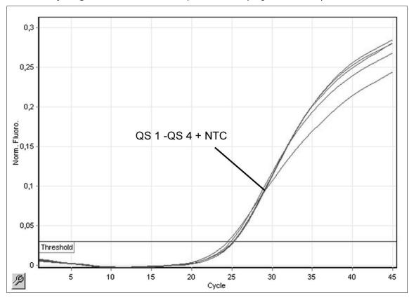
Figure 19. Detection of the internal control (IC) in fluorescence channel Cycling Yellow with simultaneous amplification of the quantitation standards (CMV QS 1–4). NTC: No template control (negative control).
