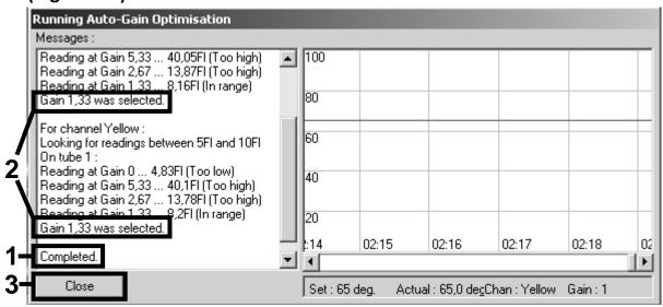
Figure 14. Gain optimization completed. Note gain values (in this case, 1.33 for both fluorescence channels).
