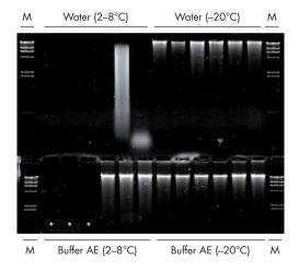
Figure 2. Agarose gel analysis of genomic DNA stored for 16 years. Agarose gel analysis (0.8% agarose gel, 1x TBE buffer, 90 V, 75 minutes) of approximately 500 ng DNA from 24 samples was performed. DNA was eluted in Buffer AE or water, and stored for 16 years at 2–8°C or –20°C. M: Marker ( $\lambda$  HindIII).
