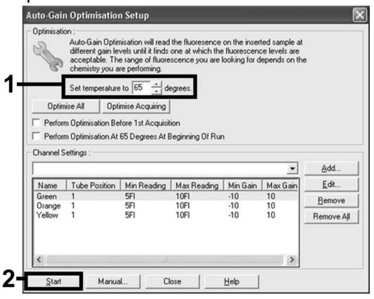
Figure 10. Adjusting the fluorescence channel sensitivity.
