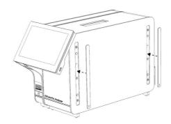
Figure 4. Reattaching the protective covers.
