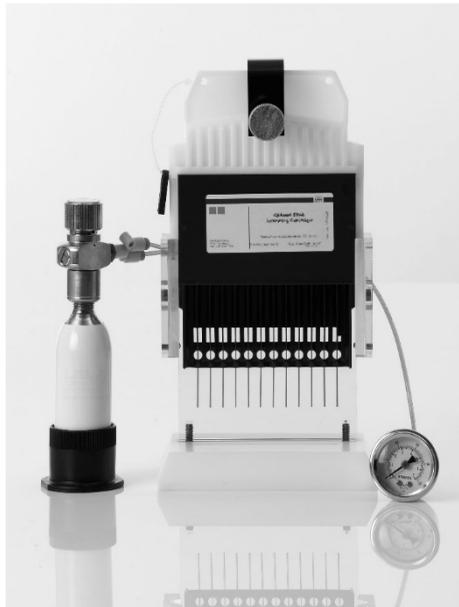
4. Slowly adjust the pressure to 60–65 psi, monitoring the pressure displayed in the pressure gauge.
