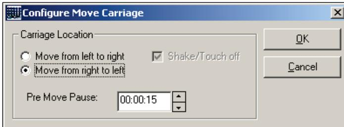
A pre-move pause (in seconds) specifies a pause that allows the dissipation of the vacuum applied to hold the carriage in place.
