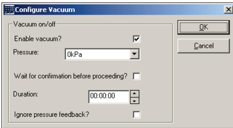
When the vacuum is to be applied, the **Enable vacuum?** option is selected and the vacuum pressure is entered.
