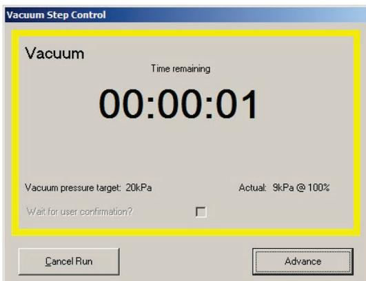
If no user confirmation is required to complete the step, the dialog box closes when the remaining time falls to 00:00:00. The vacuum operation terminates automatically, and the run proceeds without user intervention.
