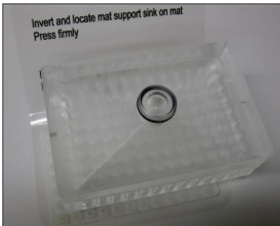
5. Align the waste sink/mat support with the silicone mat.
