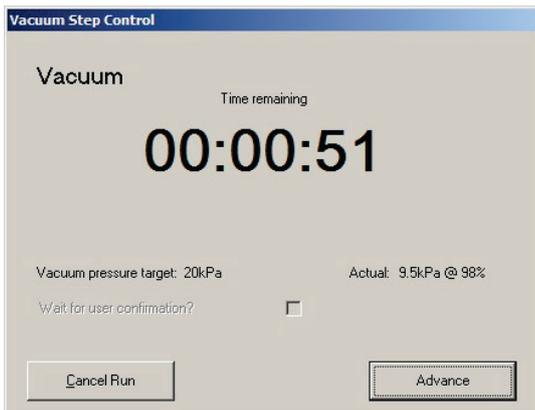
When the time remaining falls below 3 seconds, the dialog provides a visible alert.
