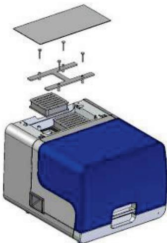
1. Remove the access hatch by pulling it.
