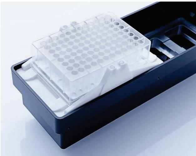
14. Gently twist the capture plate to secure it in the correct position.
