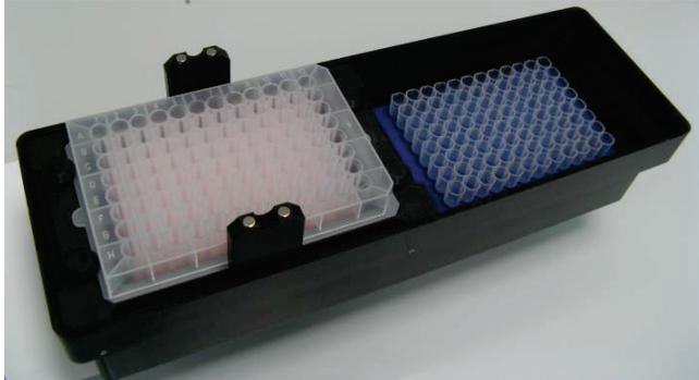
7. Place the riser block EMTR in the right (elution) side of the vacuum chamber with the pin of the riser block EMTR in the right top position.
