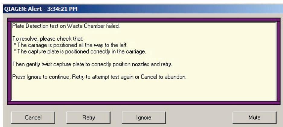
**Note:** The lid sensor is disabled during the Plate Detection test, allowing the lid to be raised and the capture plate alignment to be manually adjusted while the vacuum pump is operating during this phase of processing.
