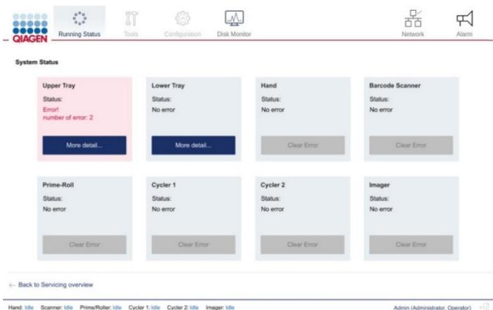
**Figure 6.** System status environment on the QIAcuity Eight after an error occurs.
