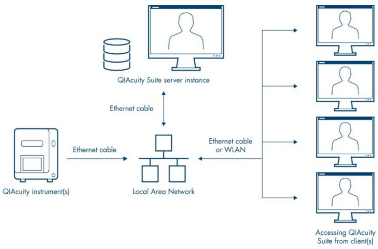
**Figure 3. The QIAcuity instrument(s) and QIAcuity Software Suite are installed to a network, allowing multiple clients to access the QIAcuity instrument(s) via a single QIAcuity Suite server.**
