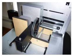
10. Move the pipettor head to the right and remove the transport lock from the worktable.
