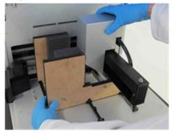
11. Unscrew the Z-axis locking screw. When this screw is removed, the pipettor head will drop to its lower position.
