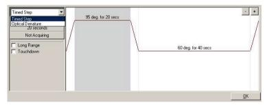
Click on the drop-down menu and select **Optical Denature**. The temperature and hold time are removed and the **Optical Denature** icon is displayed.
