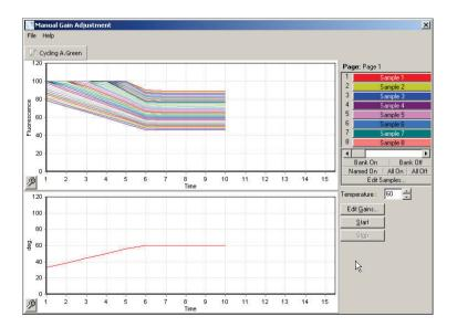
By default, all samples are shown in the display. Samples can be removed from or added to the display using the toggler to the right. The toggler consists of colored cells, each of which corresponds to a sample in the display. Samples with a brightly colored cell are displayed, while samples with a faded cell are not displayed. Samples can be switched on or off by clicking on the cell or by dragging the mouse pointer across several cells at time.
