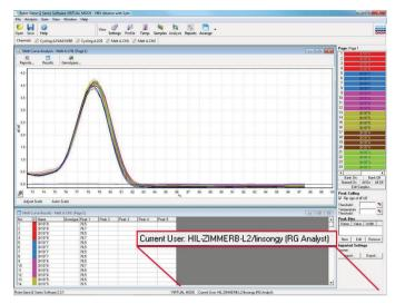
7. By logging in as an administrator again, RG Operator rights can be assigned to **linsongy** and the RG Analyst rights can be removed again. Then, the software needs to be launched again. This time, the **Analysis** menu and **Reports** button are missing, and the Run menu is enabled. The status bar indicates that the user **linsongy** belongs to the RG Operator group.
