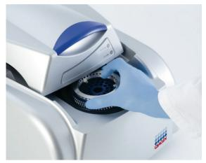
6. Close the lid and set up the run profile using the Rotor-Gene Q software.
