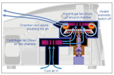
Illustration of the heating and cooling system.
