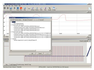
This can be used to monitor who has modified the contents of a file. The Security Audit Trail Detail contains more detail, such as the unique identifier of the user. This identifier is important to avoid a user creating an account with the same name on another computer and thereby impersonating another user. In this case, the usernames will be the same, but the account IDs will be different.
