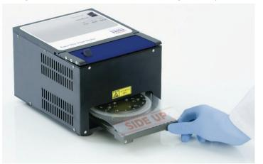
8. To activate the sealing mechanism, first press down on the blue anodized bar at the top of the Heat Sealer, then push back the black catch.
