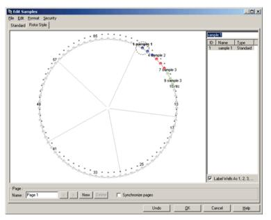
The **Rotor Style** tab provides a cutdown version of the **Standard** tab and is designed for users who want to setup sample names and colors quickly. It is not possible to define some settings, such as the whether the sample represents a standard or the known concentration of each standard, in this tab. If these need to be defined, the standard tab should be used.
