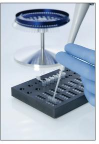
2. Place the Caps securely on the Strip Tubes and visually inspect to confirm a tight seal.
