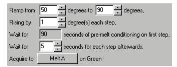
When running a standard melt the temperature is increased by increments of 1°C, waiting for 5 seconds before each acquisition. The Rotor-Gene Q MDx can be configured to perform melts in 0.02°C increments. The minimum hold time between temperature steps varies depending on the number of degrees between each step.
