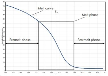
A typical HRM plot. The melt curve plots the transition from the high fluorescence of the initial premelt phase, through the decrease in fluorescence of the melt phase, to the basal level of fluorescence at the postmelt phase. Fluorescence decreases as DNA intercalating dye is released from dsDNA as it melts into single strands. The midpoint of the melt phase, at which the rate of change in fluorescence is greatest, defines the melting temperature (Tm) of the DNA under analysis.
