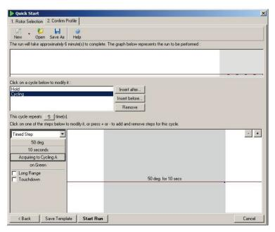
To perform EndPoint analysis, perform a profile with a hold at 50°C for several minutes, then a cycling step with 1 step (50°C for 10 s), acquiring on the required channel. Set the number of
