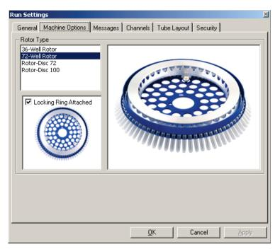
The rotor should be set to that currently installed in the Rotor-Gene Q MDx. If opening an existing run, this setting will reflect the rotor that was installed in the cycler at that time.
