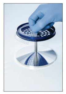
**Important**: To achieve maximum temperature uniformity, each position in the rotor must contain a tube. Filling all positions in the rotor ensures even airflow to every tube. Keep a set of empty capped tubes available that can be used to fill any unused positions.
