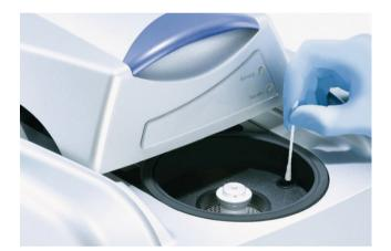
To avoid dust build up, keep the lid of the Rotor-Gene Q MDx closed when the instrument is not in use.
