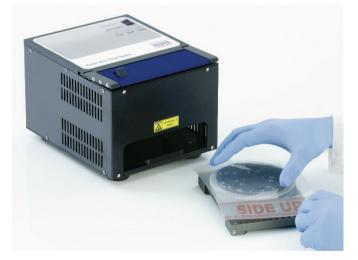
7. Slide the assembly into the Rotor-Disc Heat Sealer using the guide rails on the side of the Rotor-Disc Loading Block. Ensure that the Rotor-Disc Loading Block is pushed in completely.
