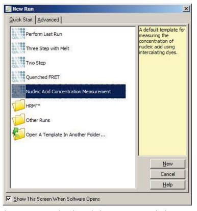
To set up the run, select Nucleic Acid Concentration Measurement from the Quick Start wizard.
