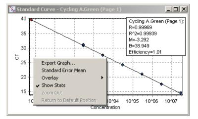
The values on the standard curve are recalculated dynamically as the threshold level is varied by clicking and dragging the threshold line in the main window. Blue dots on the curve represent the samples that have been defined as standards and red dots represent the unknown sample data points.
