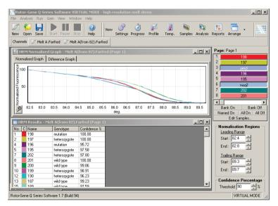
Autocalling of samples is achieved by clicking **Genotypes**. Enter the name of the genotype, followed by the sample number, which is used as a positive control to call unknown samples automatically.
