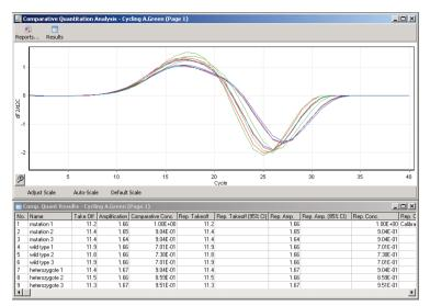
**Comparative quantitation results.** The reaction efficiency is shown in the "Amplification" column as a score out of 2 (2 = 100% efficiency).
