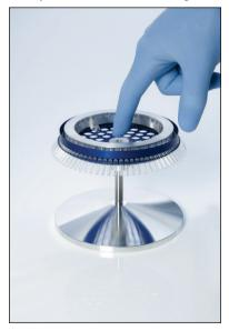
Insert the assembly into the Rotor-Gene Q MDx chamber by clicking into place using the locating pin on the rotor hub. To remove, simply push down on the rotor hub to release and pull out.
