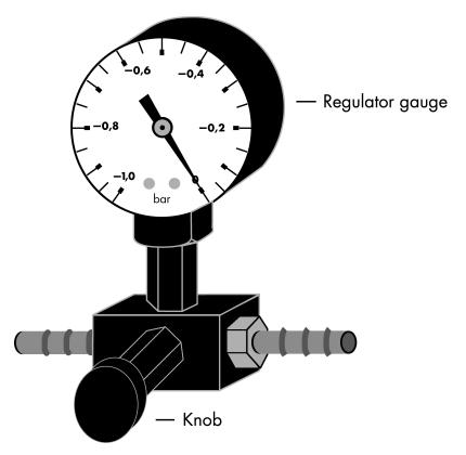
Figure 1. Schematic diagram of the Vacuum Regulator.
