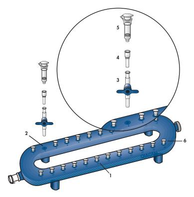
Figure 2. Setting up the QIAvac 24 Plus with QIAamp MinElute columns using VacValves and VacConnectors.
