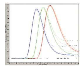
Figure 1. Robust and reproducible purification and detection of EBV in human plasma. EBV DNA was purified from 30 human plasma samples spiked at 3 different titers using the EZ1 DSP Virus Kit. EBV DNA was amplified and detected using the *artus* EBV LC PCR Kit on the LightCycler Instrument.
