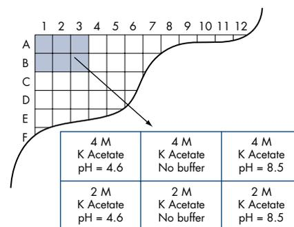
**Figure 9. Principle of Opti-Salt optimization grids.** The method involves screening of 16 different chemicals in grids of 6, where concentration of the additive and pH are varied compared to the original hit condition.
