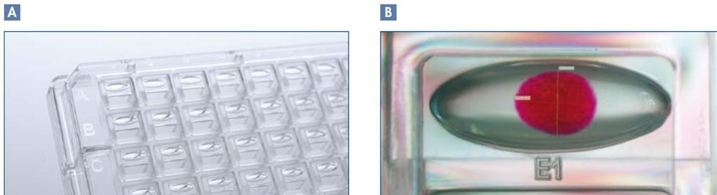
**Figure 13. NeXtal CubicPhase  $\mu$ plate.** **A** Design of precoated NeXtal CubicPhase  $\mu$ plate. **B** Top view of the oval-shaped protein well coated with monoolein (MO). For better visualization, the MO has been colored with a red dye.
