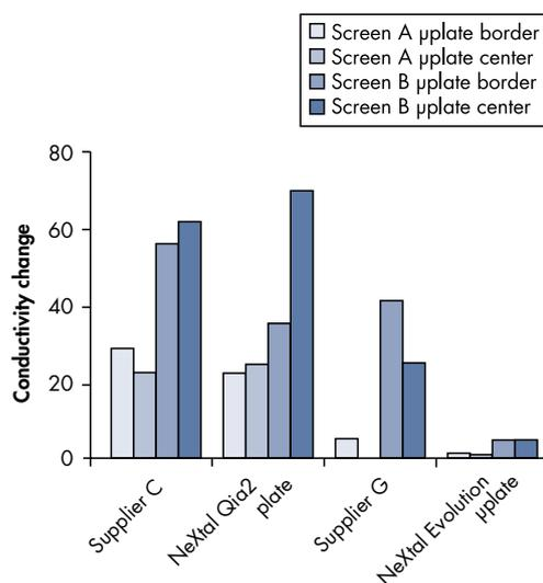
**Figure 6.** Evaporation data comparing the NeXtal Evolution  $\mu$ plate with other models. The NeXtal Evolution  $\mu$ plate ensures superior results compared to those obtained with plates from other suppliers. Screen A: 0.1 M Tris, pH 8.5, 35% MPD, 0.2 M ammonium sulfate; Screen B: 0.1 M sodium cacodylate, pH 6.5, 35% isopropanol, 0.2 M magnesium chloride. Solutions were pipetted on central or border wells of the microplate.
