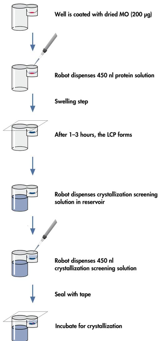
**Figure 14. Workflow for setting up a crystallization experiment using the NeXtal CubicPhase  $\mu$ plate.** The membrane protein solution is dispensed directly onto the dry lipid (monoolein). The protein solution diffuses into and rehydrates the lipid, resulting in the passive formation of the lipidic meso phase.
