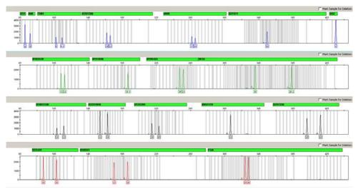
Figure 27. Reaction stability for 16 hours incubation at room temperature. PCR samples were incubated at 20°C for 16 hours in between the PCR pipetting step and the start of the thermocycler. 500 pg DNA 9948 were used as template.
