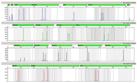
Figure 11. Electropherogram of 500 pg control DNA 9948 amplified in the presence of 500 µM hematin.
