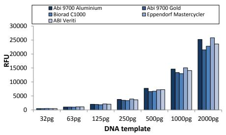
Figure 7. Performance on different PCR thermal cyclers. Different amounts of control DNA 9948 were used as, as indicated in the figure. Each sample was run in duplicate. A standard 30-cycle protocol was used. Average peak heights across all markers are shown.
