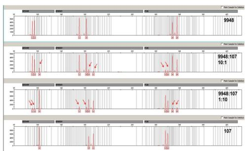
**D**. Expected bp positions of uncovered minor component peaks are indicated by red arrows. D2S441: Heterozygote + homozygote, no overlapping allele, the three non-overlapping minor component peaks can be assigned. D18S51: Heterozygote + heterozygote, no overlapping allele, three minor component peaks can be assigned, one minor component peak is overlapping with stutter position. FGA: Heterozygote + heterozygote, no overlapping alleles, all minor component peaks can be assigned.
