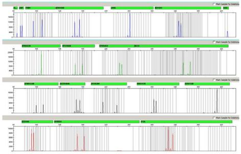
Figure 17. Electropherogram of 500 pg control DNA 9948 amplified in the presence of 0.5% ethanol.
