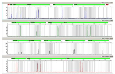
Figure 6. Reduction of PCR cycle numbers with elevated template DNA amounts. Results for amplification of 2.5 ng control DNA 9948, using a total of 24 instead of the standard 30 PCR cycles. The template amount of the Quality Sensor is optimized for 30 cycles, thus reducing the cycle number reduces the QS signals detected.
