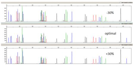
Figure 1. Influence of MgCl2 concentration. Fast Reaction Buffer 2.0 (FRM 2.0) was supplemented with different concentrations of MgCl2 matching the specification of production, or 30% higher or lower. Representative electropherograms of sample quadruplicates are shown.
