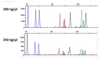
**Figure 19. Effect of high levels of collagen.** 500 pg of control DNA 9948 was amplified in the presence of 200 ng or 250 ng/µl collagen. Arrows indicate PCR products showing split peaks caused by partial adenylation.
