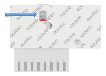
Figure 23. Sample inspection window (blue arrow).
