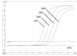
Detection of the quantitation standards (HI Virus-1 RG QS 1–4) in fluorescence channel Cycling Green. NTC: No template control (negative control).
