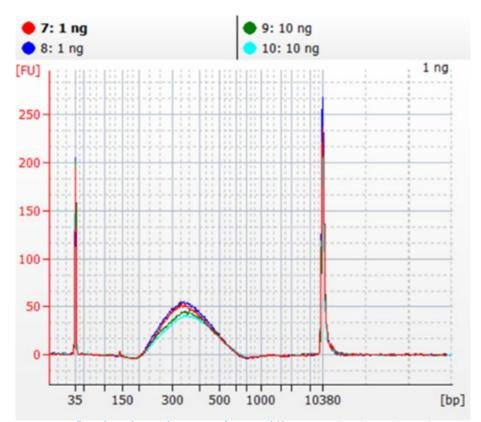
Figure 3. Capillary electrophoresis device trace of generated libraries. Capillary electrophoresis device trace data showing the correct size distribution of library fragment and the absence of adapters or adapter-dimers. Shown are replicate libraries starting from 1 ng or 10 ng bisulfite-converted DNA. Library of 1 ng was amplified for 14 cycles and 10 ng library was amplified using 10 cycles of PCR. Libraries were diluted 1:10 and loaded on an Agilent High Sensitivity DNA chip.
