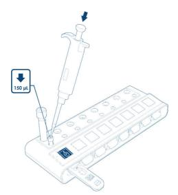
8. Mix the contents of the QIAreach QFT Processing Tube by pipetting up and down at least 4 times. Take care to not introduce foam while pipetting.
