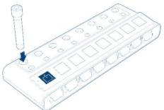
4. Remove the eStick from the packaging, label with patient identifier, and insert into the QIAreach eHub. Place the Processing Tube in the slot directly in line with the eStick.
