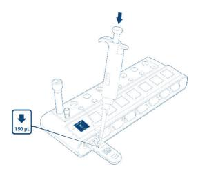
10. Following sample addition, the loading icon may appear on the eHub display for an additional 10–15 seconds before the sample is detected by the eStick. Once sample is detected, the test will start automatically, which is signaled by a countdown timer on the eHub display.
