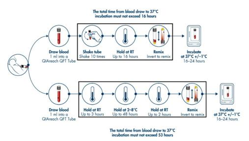
Figure 5. Blood collection and workflow options for blood directly drawn into QIAreach QFT Blood Collection Tubes (Draw Option 1).
