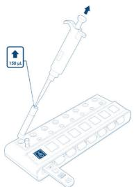
7. Add 150 µl of plasma to the QIAreach QFT Processing Tube containing the QIAreach QFT Diluent Buffer.
