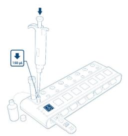
6. Remove the cap from the BCT and set aside. Carefully, remove 150  $\mu L$  of plasma from the BCT.
