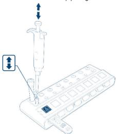
9. Remove 150 μl of sample from the QIAreach QFT Processing Tube and dispense into the sample port of the inserted eStick.
