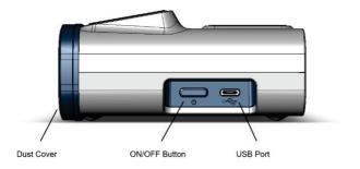
Figure 11. Side panel view of eHub with dust cover, ON/OFF switch, and USB connection port.
