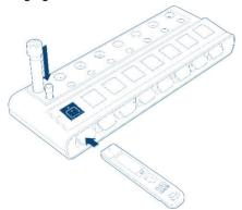
5. Add 150 µl of QlAreach QFT Diluent Buffer to the QlAreach QFT Processing Tube using a pipette.
