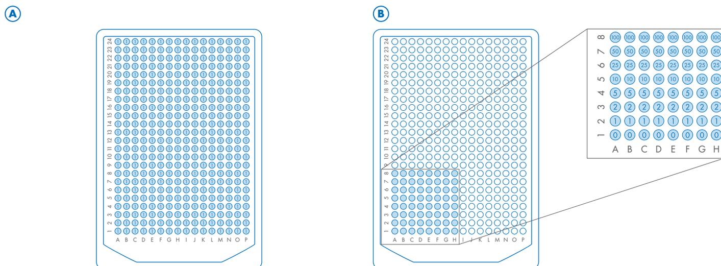
**Figure 3. Representation of the two different 384 MTP layouts set in the cellenONE X1 for cell isolation.** **A** 384 MTP layout for isolation of one single cell per well. **B** 384 MTP layout for isolation of different numbers of cells per well.
