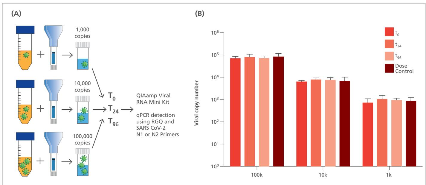
**Figure 1:** **A)** Schematic depicting the experimental setup for SARS-CoV-2 derived RNA stabilization. **B)** Quantification of RNA derived from SARS-CoV-2 0, 24 and 96 h after spike-in in PAXgene Saliva stabilizing solution. Experiments were performed in four biological replicates with three technical replicates each; data is represented as mean  $\pm$  SD.
