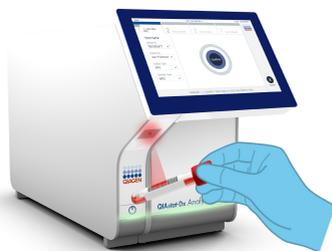
**Figure 24.** Scanning sample ID bar code.
