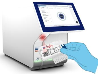
**Figure 25. Scanning QIAstat-Dx SARS-CoV-2/Flu A/B/RSV Panel Cartridge bar code.**
