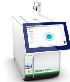
**Figure 28. Inserting QIAstat-Dx SARS-CoV-2/Flu A/B/RSV Panel Cartridge into QIAstat-Dx Analyzer 1.0.**
