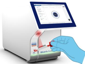
**Figure 11. Scanning sample ID bar code.**
