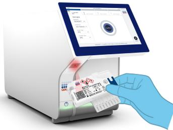
Figure 12. Scanning QIAstat-Dx SARS-CoV-2/Flu A/B/RSV Panel Cartridge bar code.
