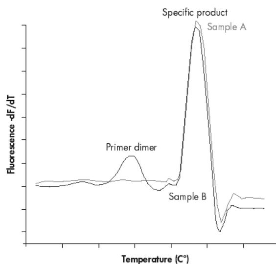
**Figure 6. Dissociation curve analysis.** Dissociation curve analysis of 2 samples (A and B). Sample A yields only one peak, resulting from the specific amplification product (primer–dimers not coamplified). Sample B shows a peak from the specific product and a peak at a lower temperature from amplification of primer–dimers.
