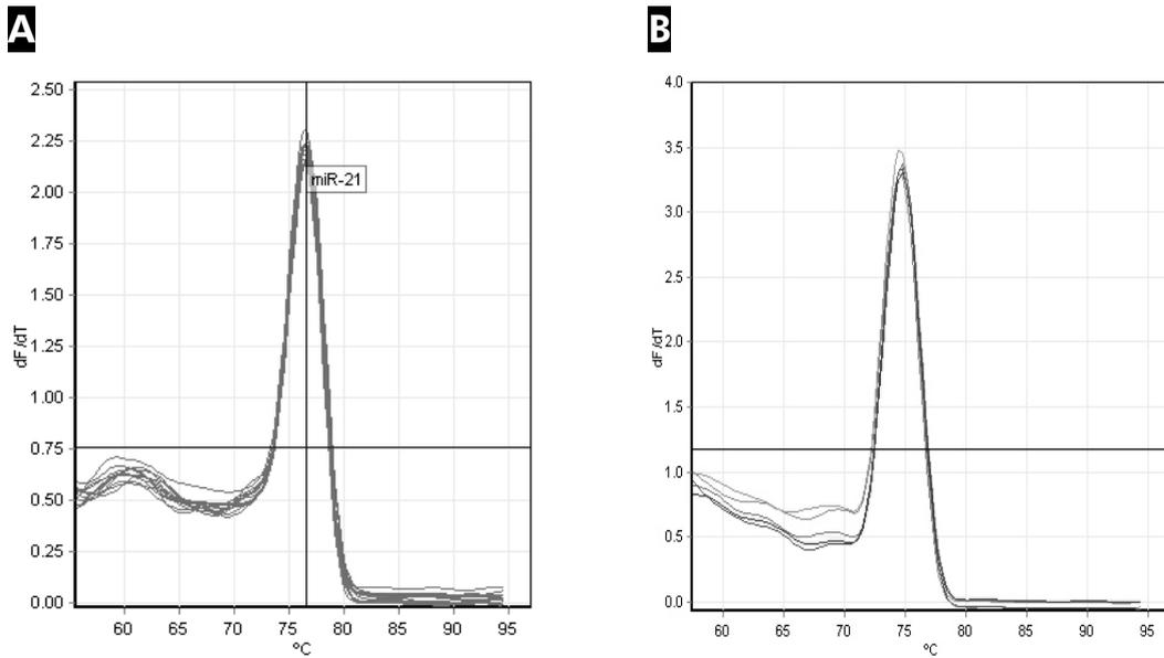
**Figure 7. Dissociation curves.** **A** Dissociation curve analysis of mature miRNA miR-21 PCR products showing single peaks from the specific amplification products. **B** Dissociation curve analysis of precursor miRNA miR-7-1 PCR products show single peaks from the specific amplification products. Dissociation curve analysis was performed using the Rotor-Gene Q.
