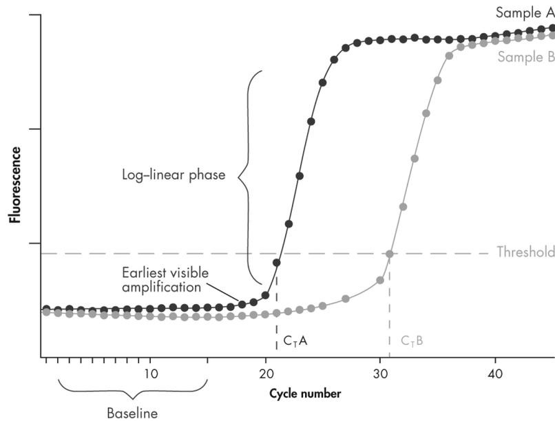
**Figure 4. Amplification plot.** Amplification plots showing increases in fluorescence from 2 samples (A and B). Sample A contains a higher amount of starting template than sample B.
