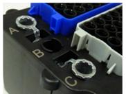
Figure 3. Microcentrifuge tube slots. Microcentrifuge tube slot B is not used in this protocol.
