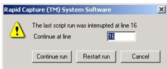
**Note:** If the instrument is powered OFF, the software will not notify the user of the line at which the last script was interrupted. The user will not see the dialog box above.
