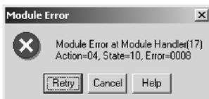
Faulty setup. Microplates were left in Stacker B from a previous run.
