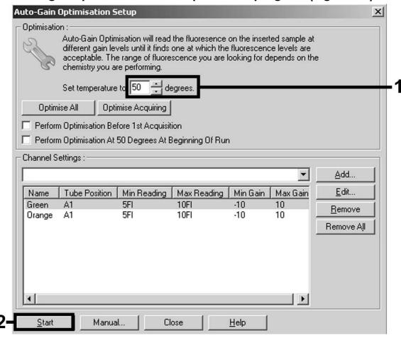
Figure 11. Adjusting the fluorescence channel sensitivity.
