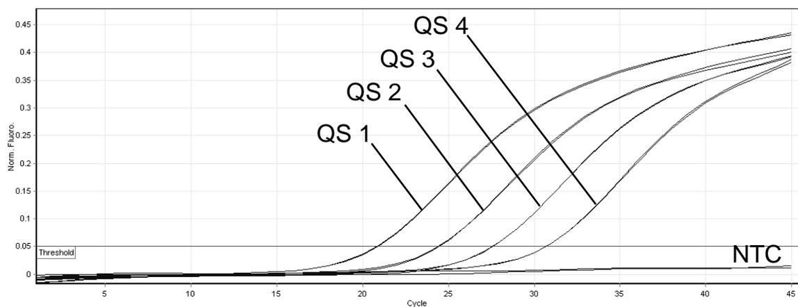
**Figure 12. Detection of the quantitation standards (BK Virus RG QS 1–4) in fluorescence channel Cycling Green. NTC: No template control (negative control).**
