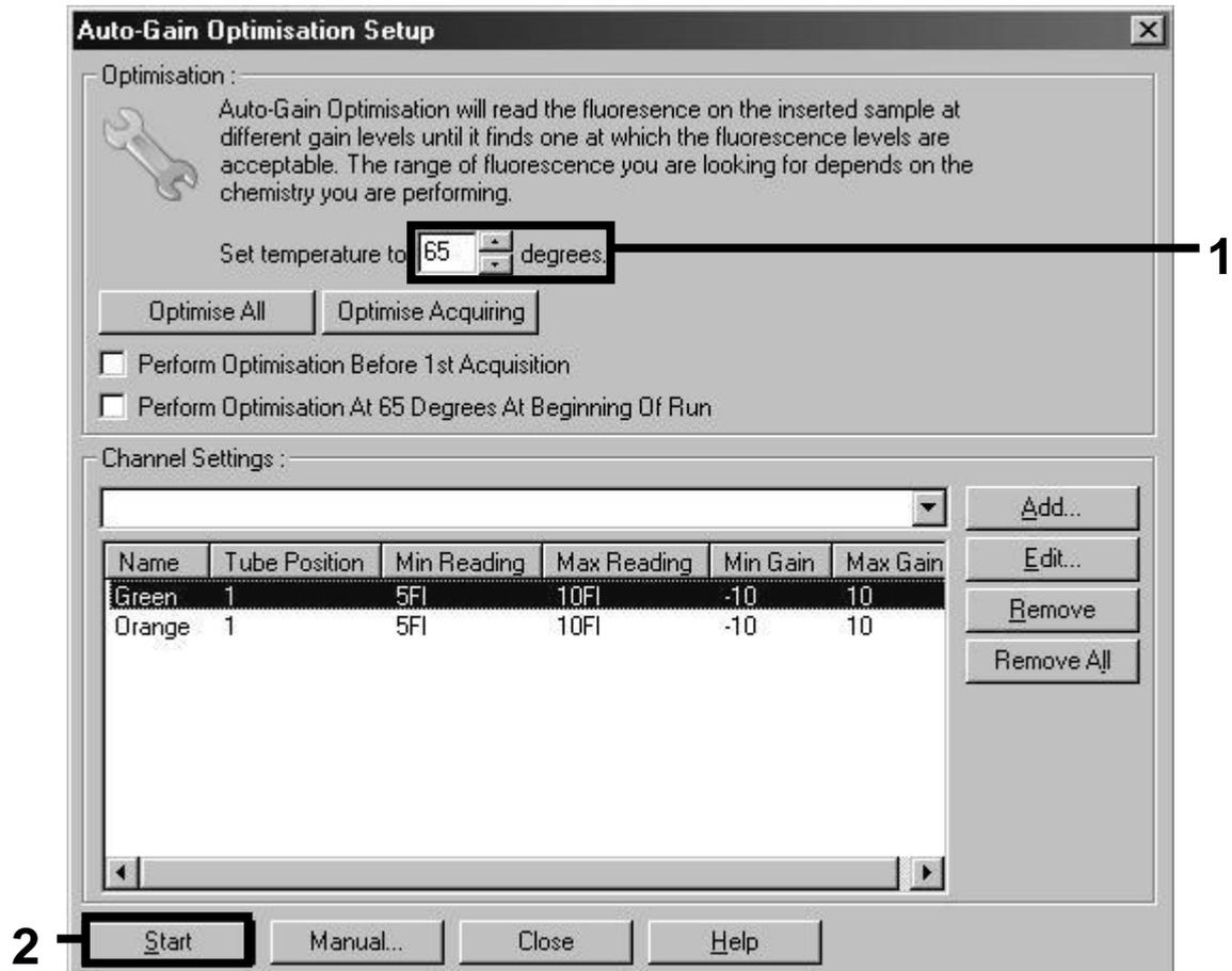
Figure 10. Adjusting the fluorescence channel sensitivity.
