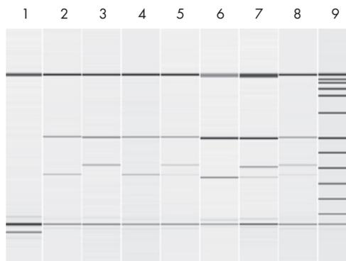
**Figure 1. CAPS analysis for the *A. thaliana* *PKS3* gene.** CAPS of the *PKS3* gene were prepared from individual *A. thaliana* plants and resolved on the QIAxcel system using the QIAxcel DNA Screening Kit.
