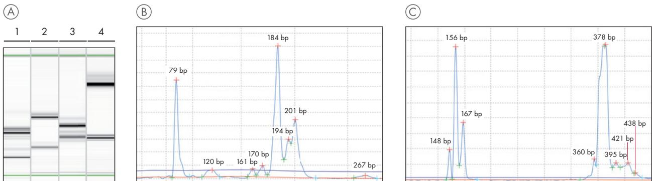
**Figure 5. Analysis of a sample containing more than 3 rice varieties.** A. Lane 1: RM1 + RM72. Lane 2: RM44 + RM55. Lane 3: RM202 + RM241. Lane 4: RM171 + RM348. B. Electropherogram of the RM1 and RM72 markers. C. Electropherogram of the RM171 and RM348 markers. With such complex allele patterns, identification requires additional analysis of physically different grains present in the sample.
