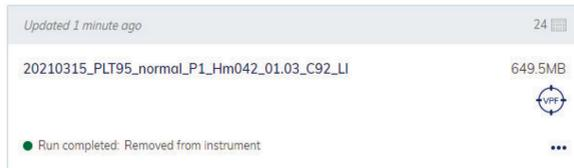
To apply the VPF to this plate, **do not** press the VPF button on the plate overview screen. Instead, please click on the plate name to open the plate in the plate configurator.
