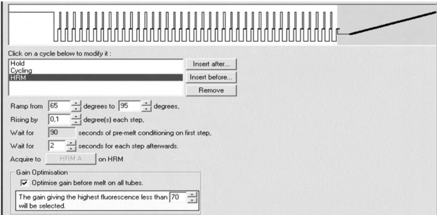
**Figure 2. Programming the Rotor-Gene system for HRM analysis.** Program the cycling protocol for gene mutation analysis described in Figure 1 and Table 2. For HRM analysis, ramp from 65°C to 95°C, rising by 0.1°C each step.
