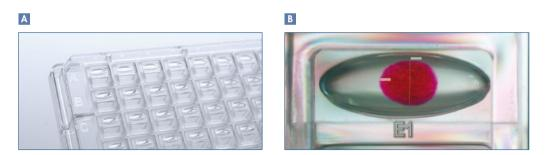
Figure 13. NeXtal CubicPhase µplate. A Design of precoated NeXtal CubicPhase µplate. B Top view of the oval-shaped protein well coated with monoolein (MO). For better visualization, the MO has been colored with a red dye.
