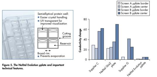
Figure 6. Evaporation data comparing the NeXtal Evolution µplate with other models. The NeXtal Evolution µplate ensures superior results compared to those obtained with plates from other suppliers. Screen A: 0.1 M Tris, pH 8.5, 35% MPD, 0.2 M ammonium sulfate; Screen B: 0.1 M sodium cacodylate, pH 6.5, 35% isopropanol, 0.2 M magnesium chloride. Solutions were pipetted on central or border wells of the microplate.
