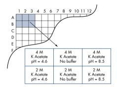
Figure 9. Principle of Opti-Salt optimization grids. The method involves screening of 16 different chemicals in grids of 6, where concentration of the additive and pH are varied compared to the original hit condition.
