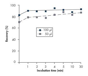
**Figure 3. Incubation time versus DNA recovery.** Using the QIAwave Plasmid Miniprep protocol, 10 µg pBluescript® DNA was purified and eluted after the indicated incubation times with either 50 or 100 µL Buffer EB. The graph shows that an incubation time of 1 minute and doubling the elution buffer volume increase yield.
