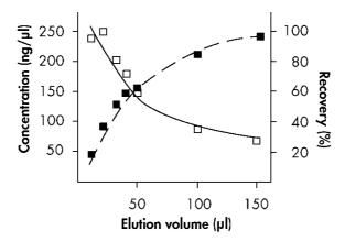
**Figure 2. Elution volume versus DNA concentration and recovery.** Using the QIAwave Plasmid Miniprep protocol, 10 µg pUC18 DNA was purified and eluted with the indicated volumes of Buffer EB. The standard protocol uses 50 µL Buffer EB for elution, because this combines high yield with high concentration. However, the yield can be increased by increasing the elution volume.
