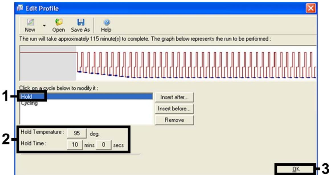
Figure 6. Initial activation of the hot-start enzyme.
